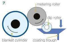
Adjustable rollers to apply more or less coating, effecting layer thickness and gloss
