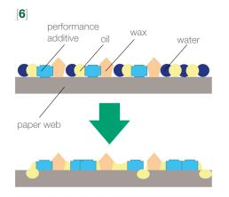
When the emulsion is being applied on the paper web, different processes will start. The water will partly evaporate and partly penetrate into the paper web, while oil particles will stay on the surface, but will also partly penetrate into the paper. On the other hand, wax and polymer will stay on the surface and build a film together with the silicone oil. **6**
